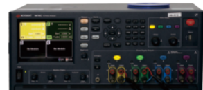
DC Power Supply Analyzer (Power Consumption Meter)
