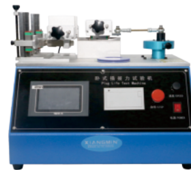
Horizontal Insertion and Removal Force Tester
