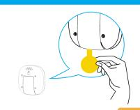
Remove battery insulation film to power on.
